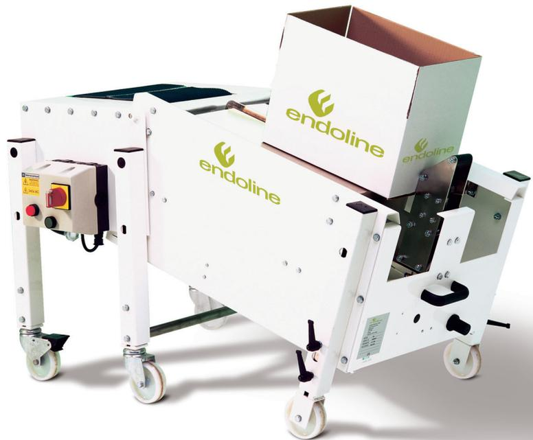
Endoline's range of case formers offers an ideal first step to packaging automation. The machines are designed to reduce the time and effort taken to manually erect a case, at a low capital cost. The machines fold the lower flaps and hold the open case steady to allow packing to take place with both hands.
