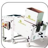
These machines can be set to an angled position, which is ideal for products that are unstable such as bags or bottles. The machine incorporates a section of horizontal belt drive so the case is horizontal at entry to the sealer.
